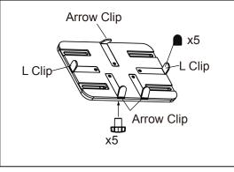
\* Stick the L CLIPS and ARROW CLIPS with PROTECT PADS and screw onto the TRAY with KNOBS.
