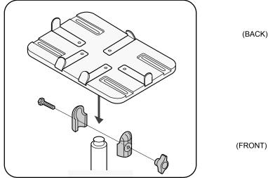
\* Screw the holding plates tightly to the ball.
