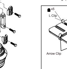
\* Stick the L CLIPS and ARROW CLIPS with PROTECT PADS and screw onto the TRAY with KNOBS.
