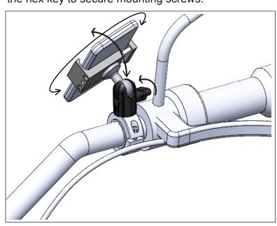
STEP 3: Adjust cellphone mount position as desired by loosing knob. Make sure every knob and screw fully tightened and secured before use.
