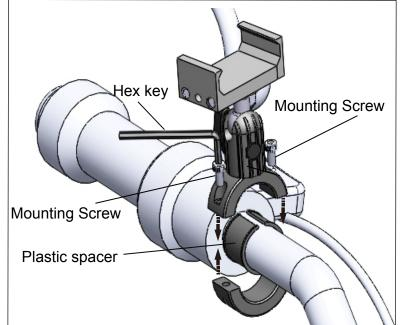
STEP 1: Choose one plastic spacer to fit handle bar. Attach mount to handle bar around spacer. Use the hex key to secure mounting screws.
