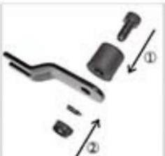
STEP A: Choose suitable link bracket, assemble with screw base, washer and screw nut.
