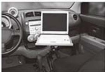
STEP 5 :After being adjusted to a suitable position, put the laptop on the tray and fasten it by velcro belt tightly.
